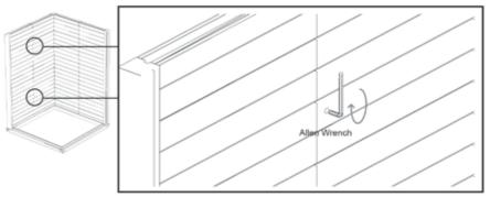
Before moving on to securing the next wall element, make sure that both cam locks are properly secured
