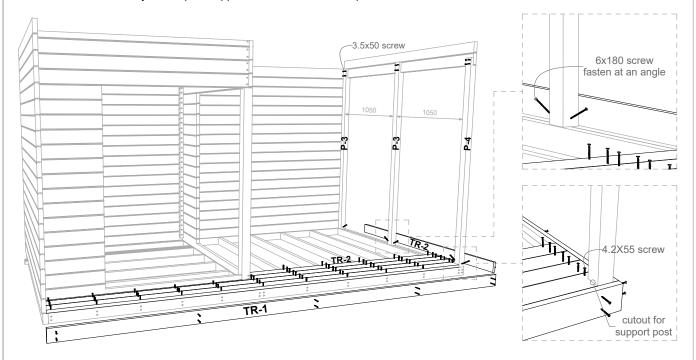
3. Make cutouts for the support posts and fasten the decking boards to the base frame using 4.2x55 screws. Cut the last decking board to width using a circular saw.
